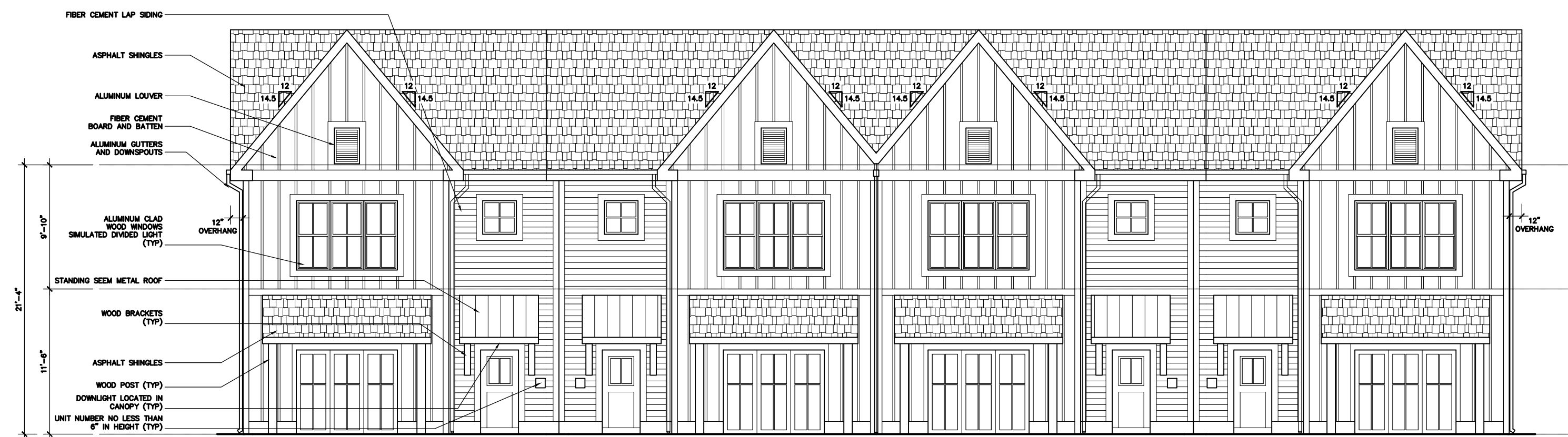
elev 5 FRONT ELEVATION 1/8"=1'-0" A201 FOUR UNIT BLDG
