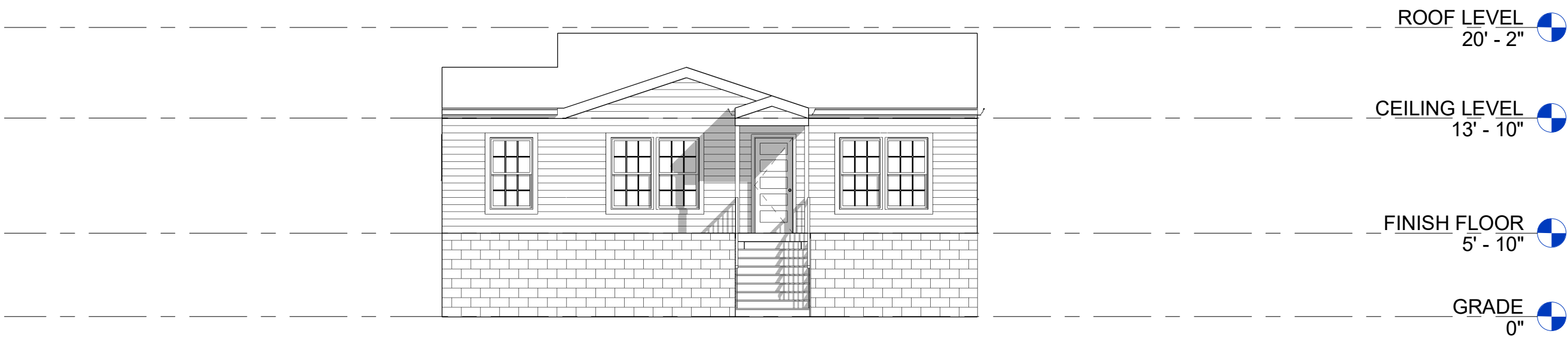
② EXISTING FRONT ELEVATION 1/8" = 1'-0"
