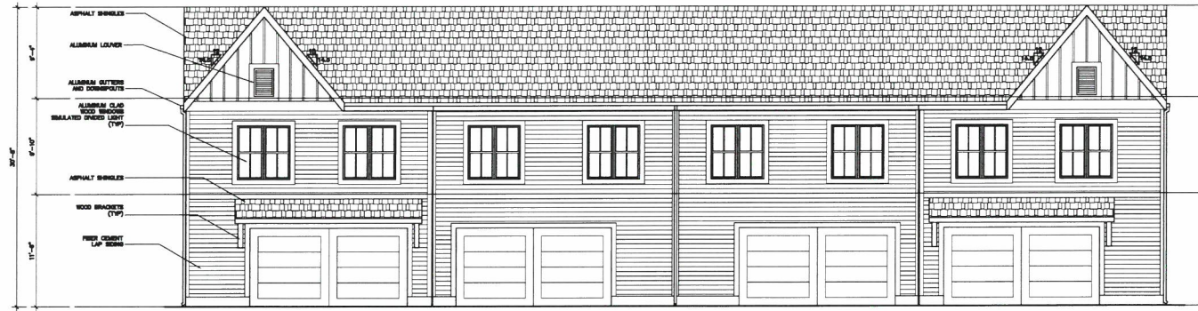
elev 7 REAR ELEVATION 1/8"=1'-0" A201 FOUR UNIT BLDG
