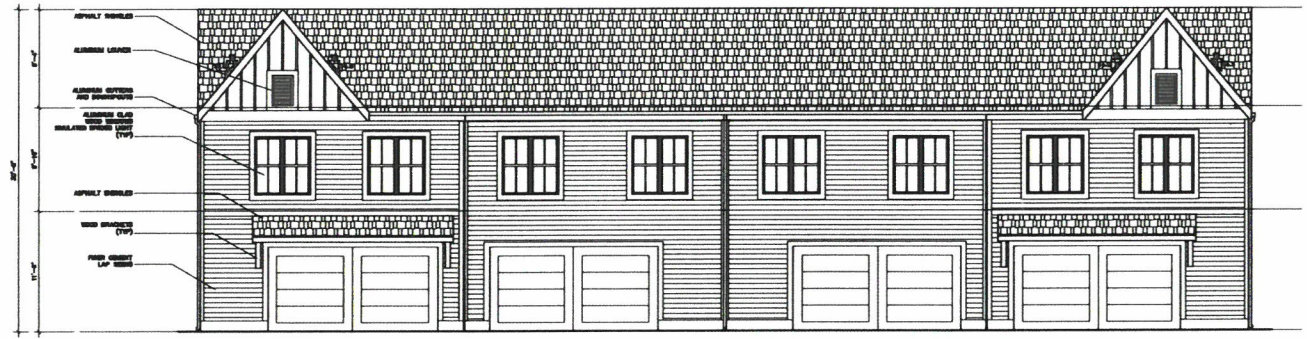
7 REAR ELEVATION FOUR UNIT BLDG
