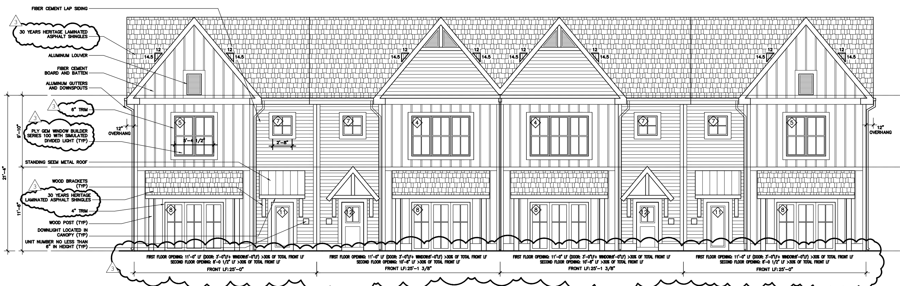
elev 5 FRONT ELEVATION 1/8"=1'-0" A201 FOUR UNIT BLDG
